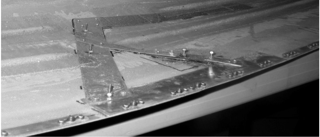
Here's the strip that encompasses the Archer antenna. This not only secures the antenna but provides your ground plane.
